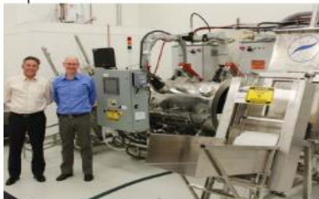
► John McMill (left) and Tim Duvant stand in front of a 20 kW vacuum microwave dryer in the EnWave pilot plant. Resistance to electrically powered processing equipment is fading, causing the transition to technologies such as vacuum microwaves. Source: EnWave Corp.
